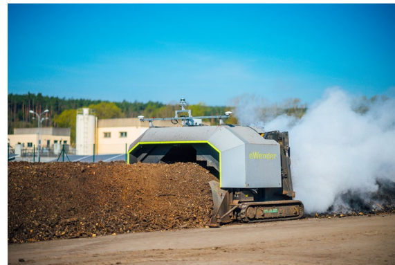
Figure 1. Prototype of an autonomous electric-powered Compost Turner working on compost windrows at an industrial plant
