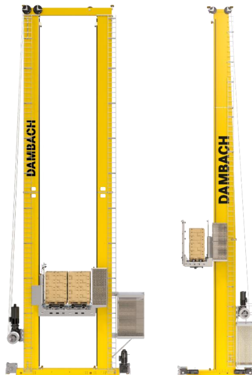
Figure 1 Example of a stacker crane (front view left, side view right). The total mass of up to 40 tons in combination with typical heights of 30 meters cause power peaks of several 100 kW. Regarding the front view, the two drives are colored in black, and the lifting gear is located at the left side and the running gear at the bottom (credit: DAMBACH GmbH & Co. KG).
