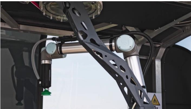
Figure 3. The suspension connects the robotic arm with the vehicle. The additional degree of freedom significantly increases the reach of robot.
