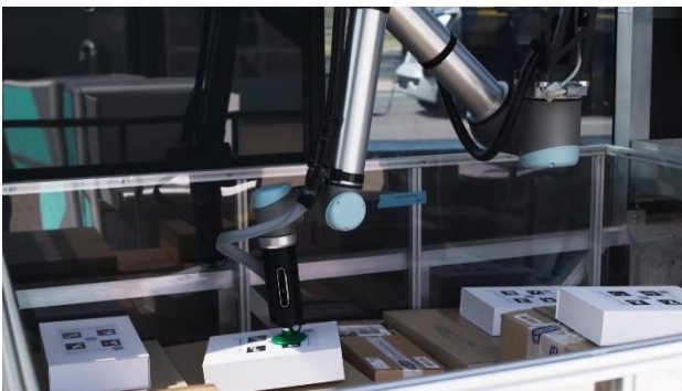
Figure 9. The robotic arm picking up a parcel to deliver it to the parcel station.
