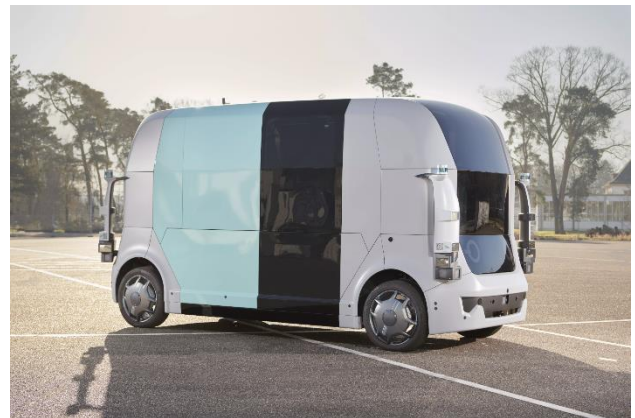
Figure 1. The autoCARGO vehicle platform combines a purpose-built level 5 autonomous car with a fully automated parcel delivery system.
