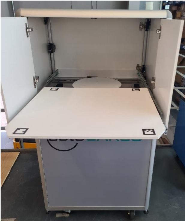
Figure 4. Model of the parcel station for demonstration purposes, which is shown with the side facing the vehicle. It is depicted in the opened and fully extended state.
