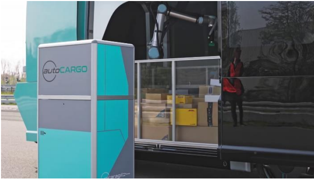
Figure 8. After the doors opened, the handling system is about to start the delivery process.
