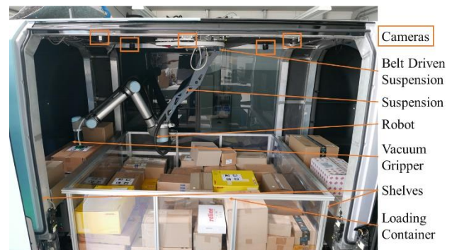
Figure 2. The interior of autoCARGO . Next to the large loading container are the shelves for parcels picked up on route. They are handled by the mounted robotic arm, which is guided using the multi-camera setup.
