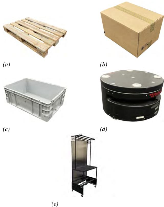
Figure 2: The objects used in Multi-log are a) pallets, b) cardboard boxes, c) small load carriers, d) mobile robots, and e) movable workstations.
