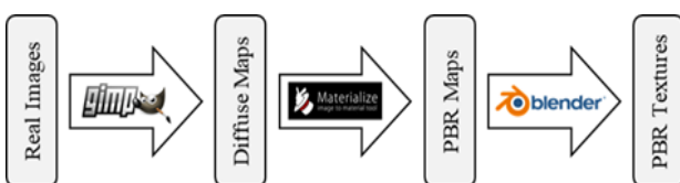
Figure 2: Workflow for creating a photorealistic model.
